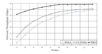
Fig. 3. Network throughput with 12 channels.
